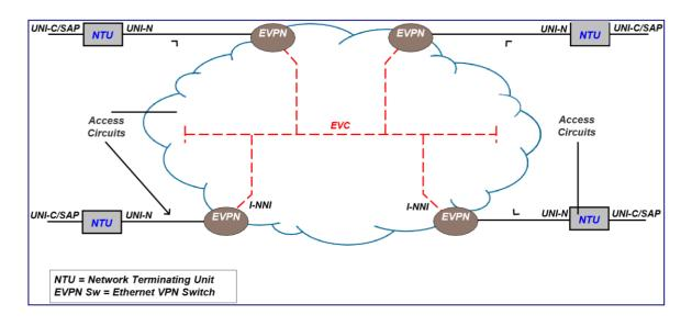
As illustrated in the above diagram, all sites have single SAP with an Access Circuit within which a contracted bandwidth may be defined. Contracted bandwidth represents a bandwidth profile configured on the Ethernet VPN ingress switch port.
