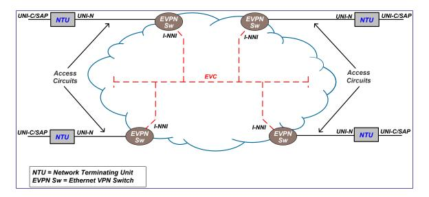
As illustrated in the above diagram, all sites have single SAP with an Access Circuit within which a contracted bandwidth may be defined. Contracted bandwidth represents a bandwidth profile configured on the Ethernet VPN ingress switch port.
